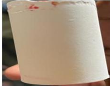
Figure 6. Defect identification through liquid penetrant test.
